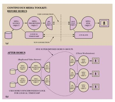
to maintain a master clock on behalf of the others. The second stack synchronizes the speeds and offsets with respect to realtime of the logical timestamp objects. To keep these values consistent, it is necessary that they be updated in the same order. Therefore, this stack is similar to the previous one, but includes a Horus protocol block that places a total order on
