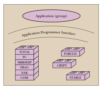
**Figure 1.** Group protocol layers can be stacked at run time like Lego blocks and support applications through one of several application programming interfaces
