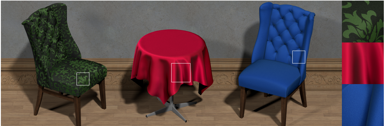
Fig. 1. Our algorithm enables fast, high-quality rendering of fabric models made up of individual fibers with multiple scattering. The table was rendered in 63 seconds, the green chair 291 seconds, and the blue chair 131 seconds on a single Nvidia GeForce GTX 970 GPU.
