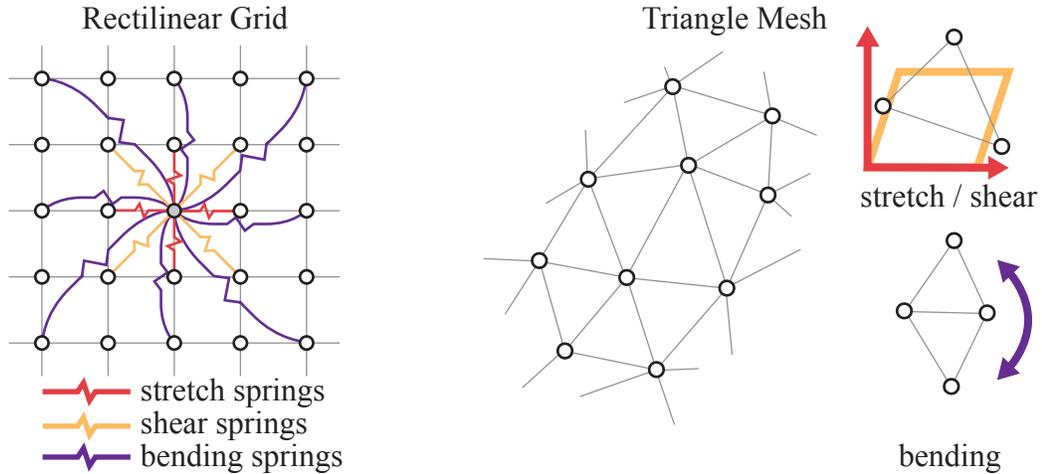
Figure 3.1: Rectilinear and triangular mesh cloth models.
