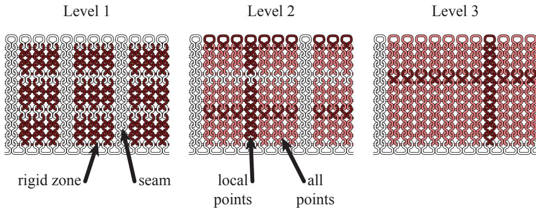
Figure 5.1: Hierarchy of zones in a simple knit
