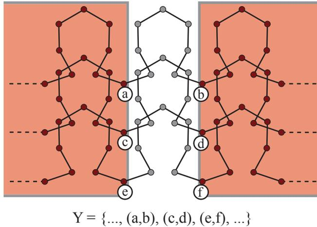
Figure 5.3: Example of intervals between rigidified zones
