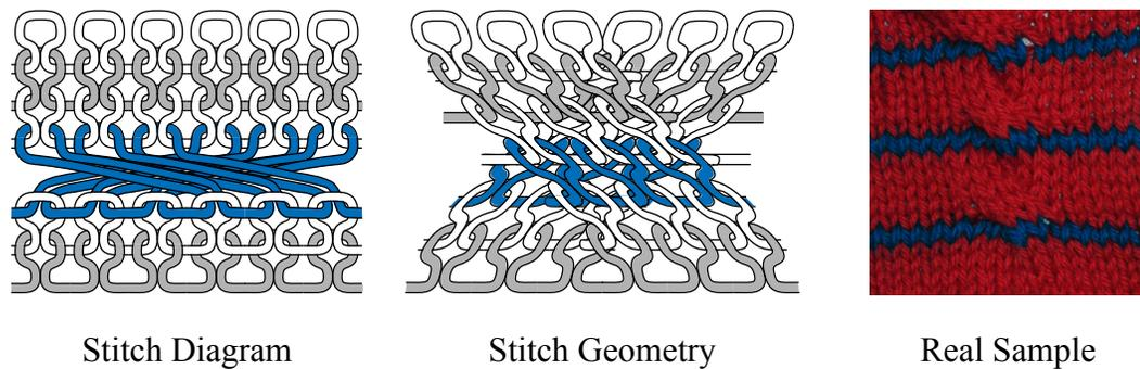
Figure 2.3: Stitch diagram, geometry, and real sample of a cable stitch
