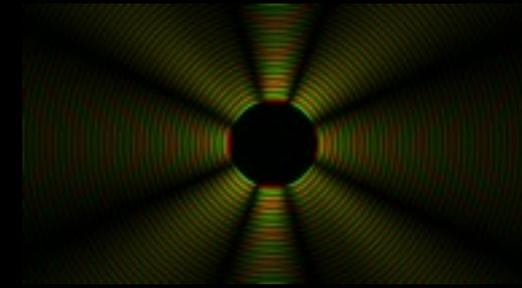
Amplitude of unit vibration:  $|p(\mathbf{x})|$
