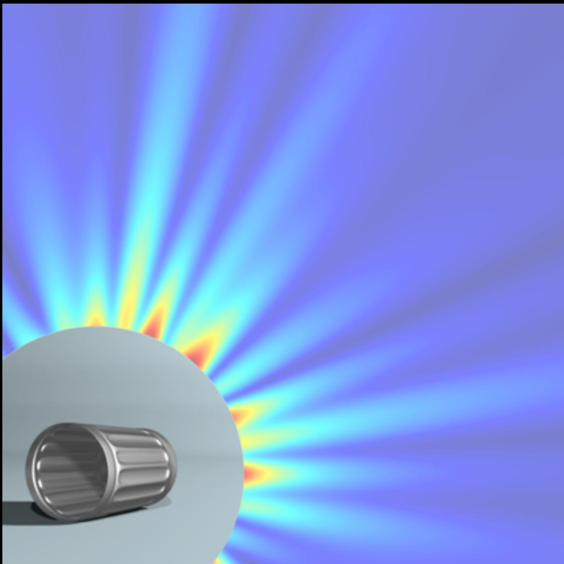
Precompute pressure samples on concentric spherical shells using fast multipole BEM
