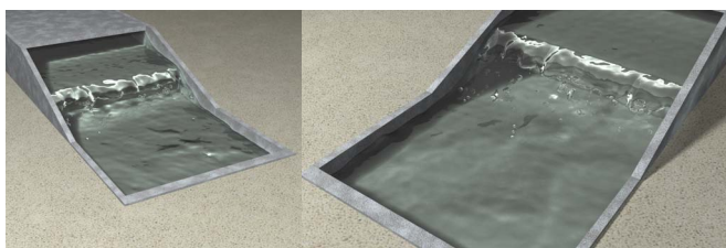
Figure 15: Water “bubbles” as it flows over a small step
